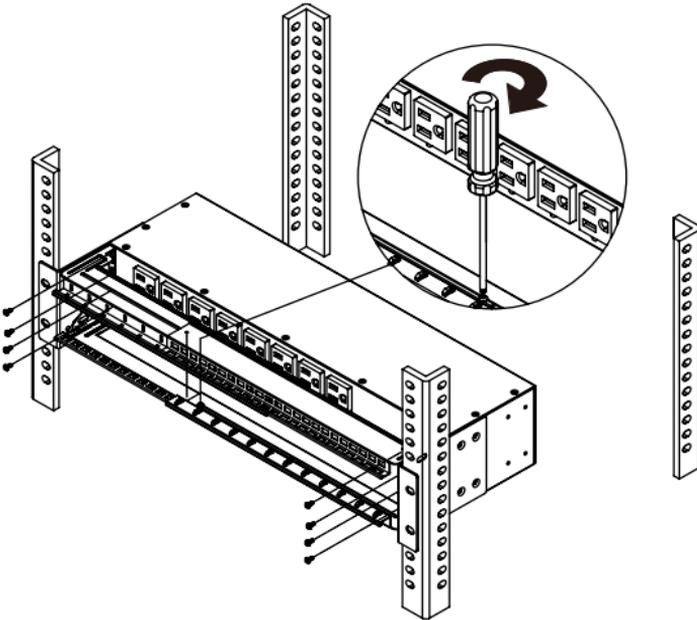
Use the provided Cable Ties to fasten each cord to the Cord Retention Tray.
