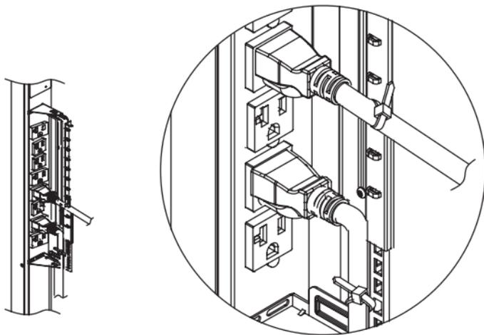
**Note:** If the PDUs are intended to install in a high temperature environment, please use the Power Cords that could sustain high temperature operation.
