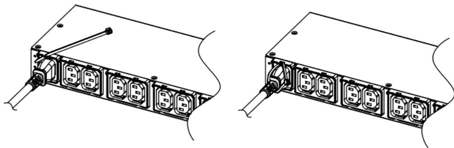
Step 2. Align and insert the Cable Tie from the bottom side of the Fixed Stand and fasten it as shown below.
