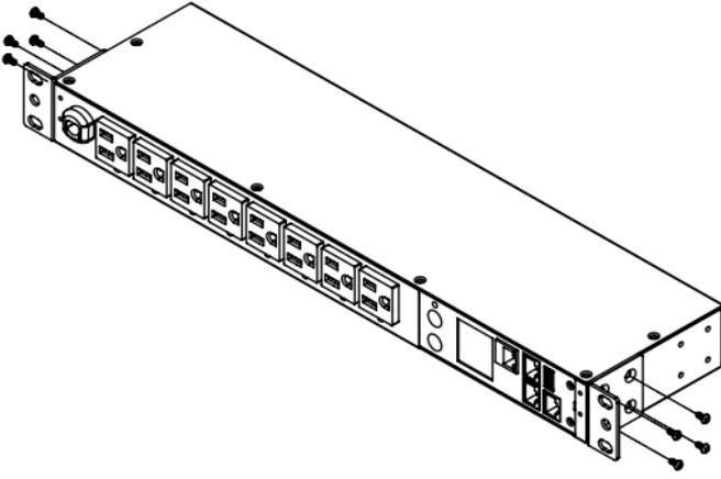
If you plan on attaching the Cord Retention Tray to the PDU, you will need to use the LONG Mounting Brackets (2).
