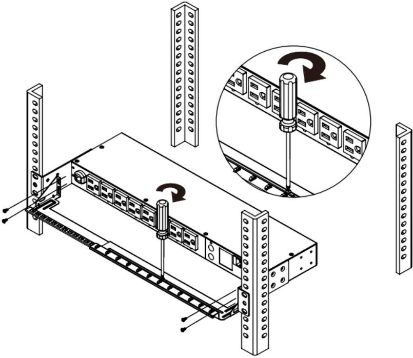
Use the provided Cable Ties to fasten each cord to the Cord Retention Tray.
