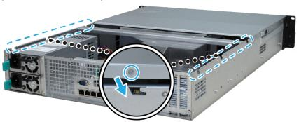
**b** Put back and fasten the screw you removed in step 2.
