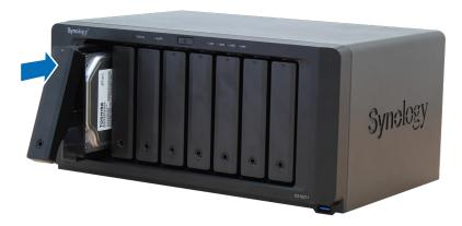
Note: Make sure that the drive tray is completely inserted. Otherwise, the drive might not function properly.
