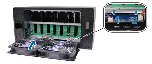
**6** Replace and tighten the four screws removed in step 3.
