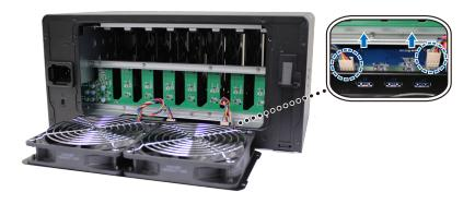
$\boldsymbol{c}\$  Remove the screws that secure the fan from the fan case.
