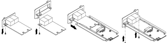
Step 1. Remove the screw holding the front panel to the card and remove the RMCARD205 front panel.
