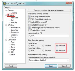
Figure 5. The PuTTY Configuration window.
