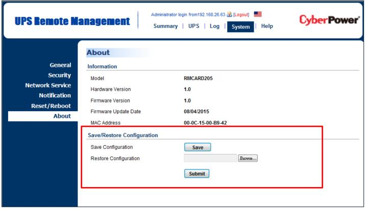
Figure 9. Save/Restore Configuration in the main window.
