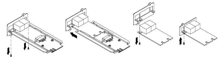
Step 1. Remove the two screws from the adapter holding the card in place.
